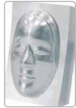
The CNC works with nano-metric resolution: In order to obtain the best part finish, the CAD-CAM coordinates should be defined with the maximum resolution possible.
